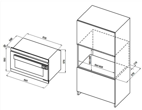
NOTE: Its installation under the table or under the baking top is not allowed (The dimensions indicated in the views are in millimeters)
