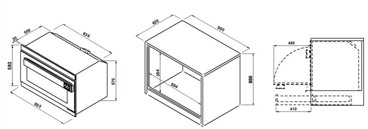
NOTE: Its installation under the table or under the baking top is not allowed (The dimensions indicated in the views are in millimeters)
