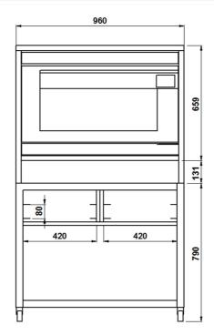
NOTE: Its installation under the table or under the baking top is not allowed (The dimensions indicated in the views are in millimeters)
