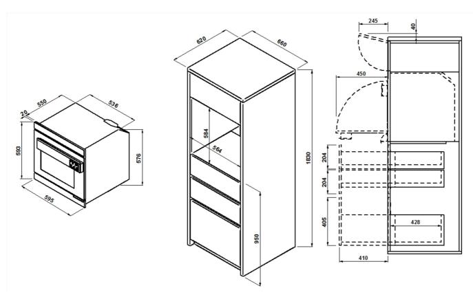
NOTE: Its installation under the table or under the baking top is not allowed (The dimensions indicated in the views are in millimeters)
