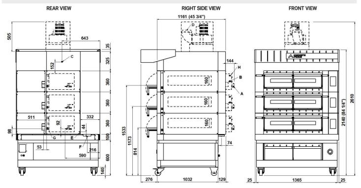
NOTE: The dimensions indicated in the views are in millimetres. \*Dimensions refer to the oversized hood.
